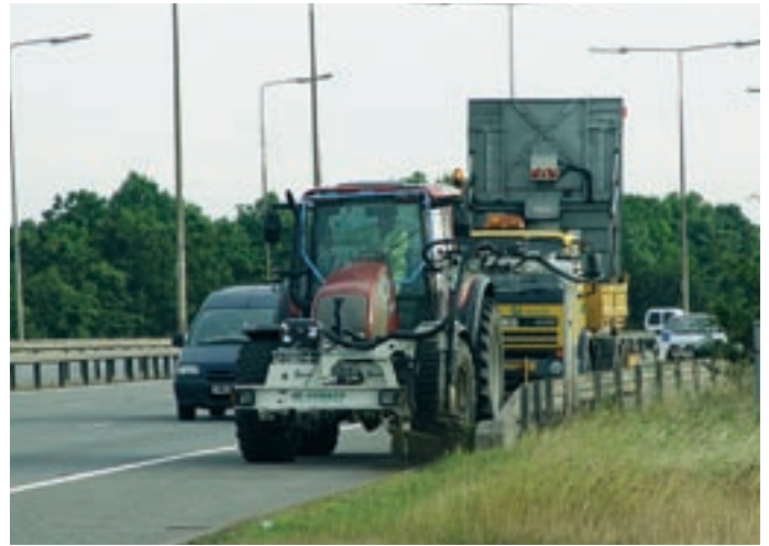
Ian White's front mounted over barrier mower is easy to operate in the dangerous environment of a motorway hard shoulder while a 50 kph transmission makes moving from site to site quick and safer.
