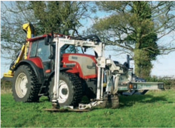
With a mower on each end Ian's drivers can undertake any operation on either side of the motorway.
