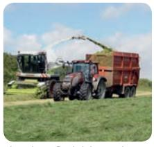
The equipment fleet includes several 12 and 14 tonnes trailers with air brakes for safety on Dorset's rolling hills. Tractors are also equipped with exhaust brakes which have cut maintenance noticeably.
