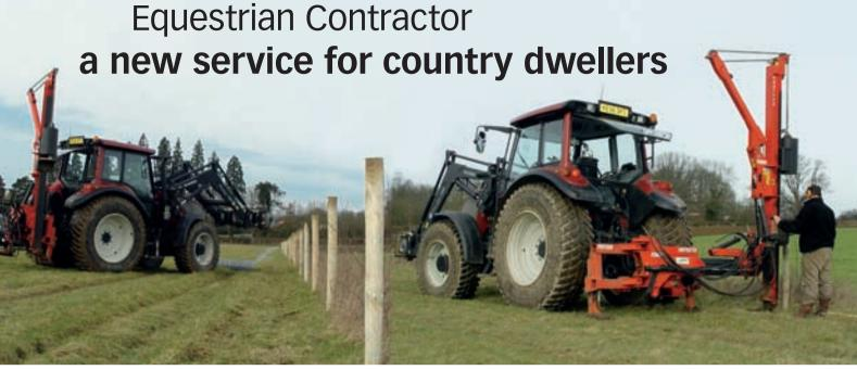
With post driver on the rear and stakes and wire on the loader there is little reason for other machines to come onto the land. James' M120 fitted with a loader and grassland tyres is ideal for fencing work
