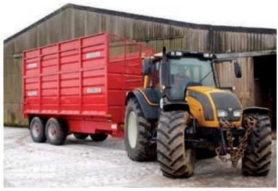
Heavy loads on busy country lanes. With air brakes, suspension and plenty of engine torque the N141 is in control and safe. The chain is usually used for recovering other machines.
