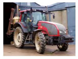
Tim's Valtra T131 equipped for spraying on narrow wheels. There is also a set of wide wheels for top work.
