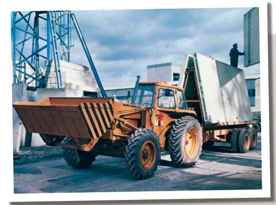
The Valmet 1100-4 was an extreme machine in 1969: 4WD, a four-cylinder turbo engine and 115 horsepower.
