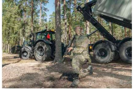
The tractors have already demonstrated their versatility with the Finnish Defence Forces. They can load and unload supplies in the forest, as well as pull containers weighing up to 16 tonnes and handle them with hook-lift trailers. In addition, tractors can be used to snow plough roads, clearing it for other vehicles.
