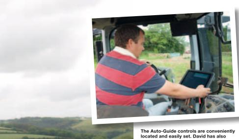
The Auto-Guide controls are conveniently located and easily set. David has also installed a TV monitor that is used in conjunction with a remote camera at the rear of balers or planters to check operations. The cab is also fitted with a hands-free mobile phone and a CB radio to keep him in contact with home and colleagues.
