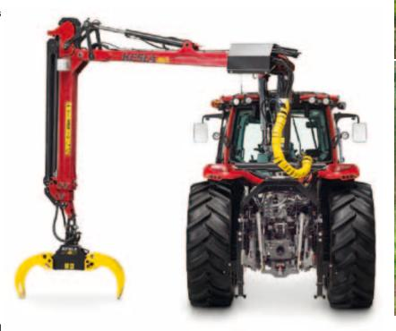
If you have to transport soil or handle fodder once in a while, then it's good to have the loader attached to the tractor. All of the hydraulic movements can be preset using the IQAN electronic control system," says Heikki.
