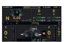
While driving all the required information can be displayed on its own screen or in four quadrants. The information displayed can be selected according to the task.
