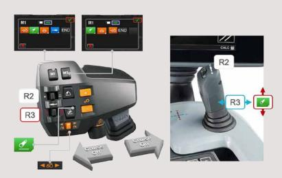
Do you want to use the U-Pilot headland management system? Programming the system is easy. You can programme sequences according to time or distance. For example, when ploughing you can programme the M1 memory button to disengage the four-wheel-drive, cruise control and differential locks, raise the plough and turn – all with a single click of the button – when you get to the headland. Similarly, you can programme the M2 memory button to do the same in reverse
