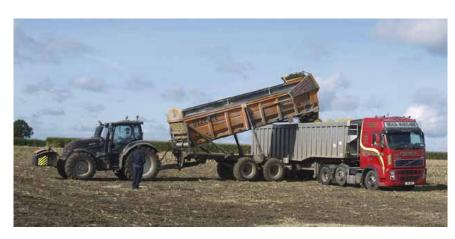
A full Dezeure self levelling trailer load of maize is transferred to the road truck. Control of the unloading is remote allowing the tractor driver to act as banksman for the truck driver.
