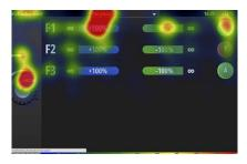
The eye movements of testers were tracked while using SmartTouch using special cameras, allowing developers to see whether users found the functions they were looking for and understood the icons.
