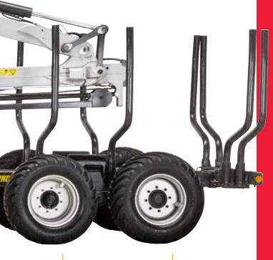
Available with hydraulic Robson drive or wheel motors Disc or drum brakes with negative handbrake
