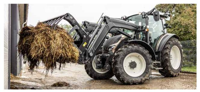
The G Series weighs 5140 kg. The light weight, compact size and agile performances makes it ideal for farm tasks. The maximum total weight is 9500 kg.
