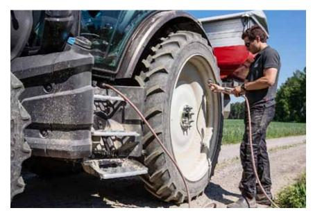
The new G Series Is available with a compressed air connector on the side of the tractor by the cab steps, making It easy to adjust tyre pressures, for example.
